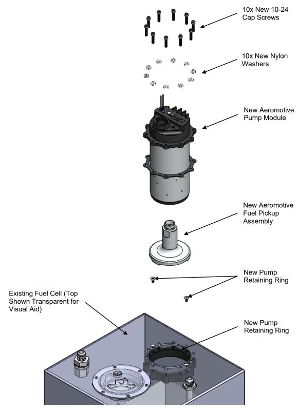
This product is intended to be installed and utilized for pump module replacement or upgrade of existing Aeromotive fuel pumps mounted on fuel cells which have already been plumbed and wired. If you are trying to install a pump module into a new cell or are replacing a non-Aeromotive pump, please contact the Aeromotive Tech Department for assistance with installation.
