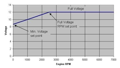
24. The initial pump voltage at idle or minimum voltage may also be adjusted by using a small screw driver and turning the "MIN VOLTS" screw on the front of the controller. Turning the adjustment screw counter-clockwise will decrease the initial pump voltage and clockwise will increase the initial pump voltage. This adjustment screw has a 15-turn range.
