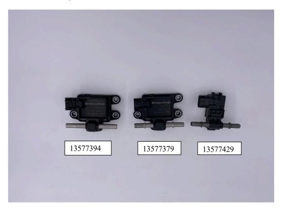
13577394 needs to be trimmed to 3.75" so 1.875" from the center of the sensor.
