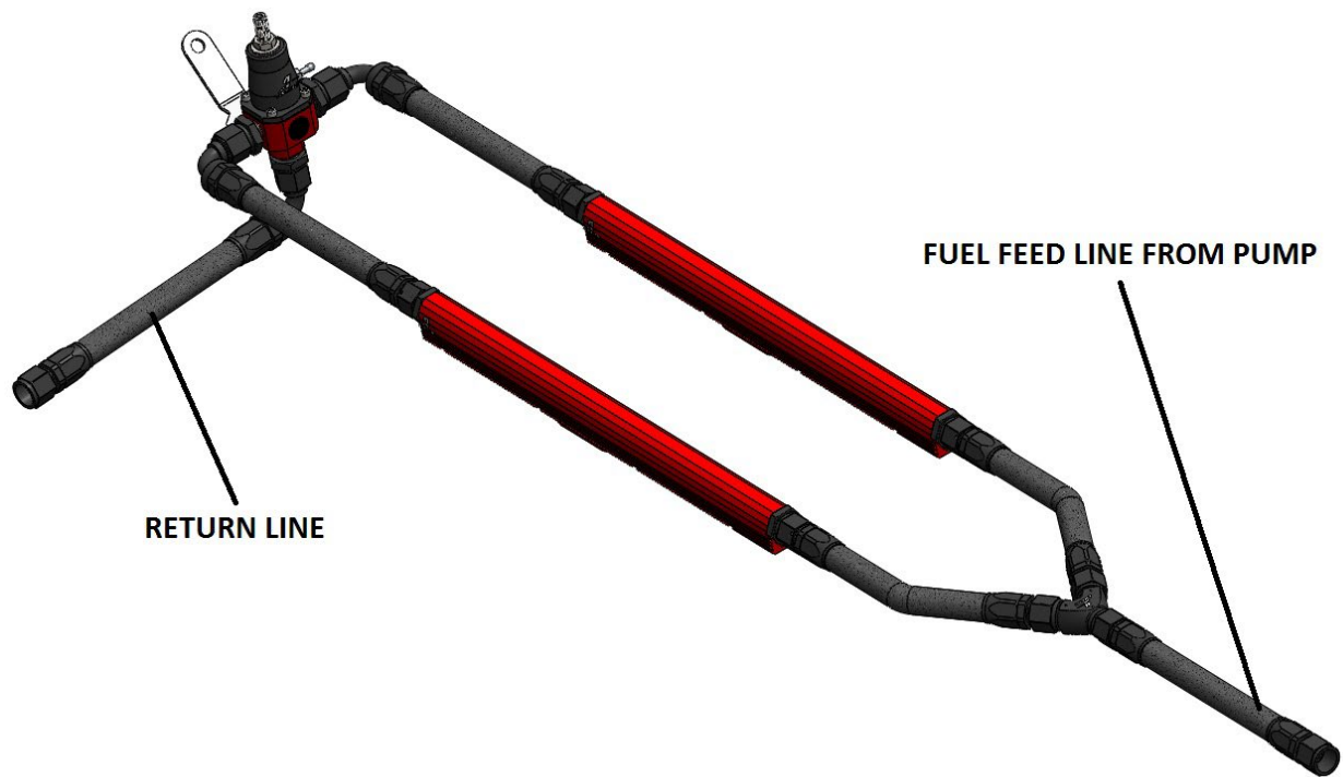
Dual Fuel Rail (Ideal Flow-Through) EFI Plumbing
