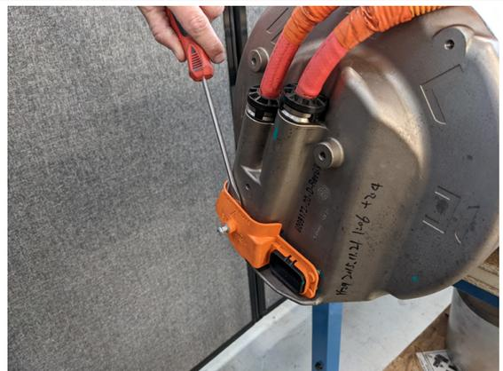
Use T-10 Torx to remove the inverter connector mounting screws.
