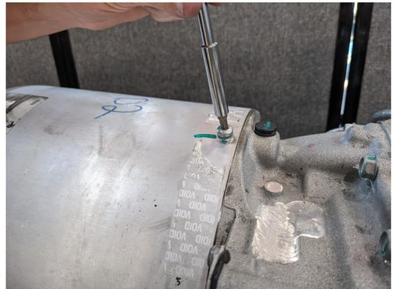
Gently move the end of the cover up/down & left/right to release it from the sealing o-ring. While doing this, give attention to also disengage the inverter connector from the end of the cover. Once fully released, completely remove the cover by sliding it straight off.
