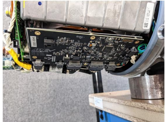
Align the screw holes and install the mounting screws. Be sure to tighten the one shield mounting screw. Double check that all connectors have been plugged in.
