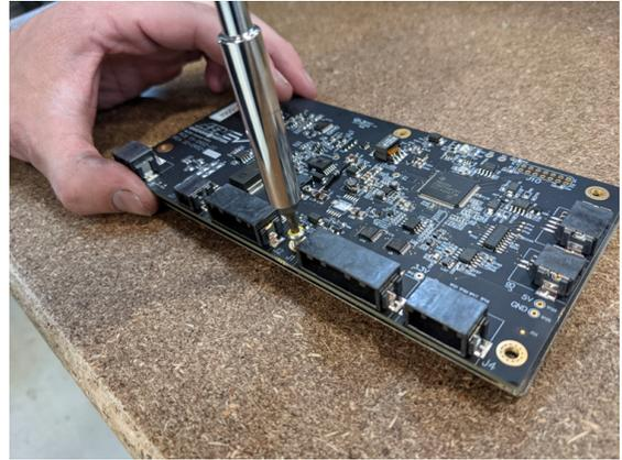
Position the Control Board back in the inverter and plug in connectors to hold it in place.
