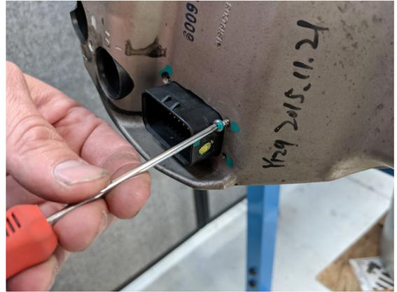
Use 13mm socket to remove HV cable mounting bolts.
