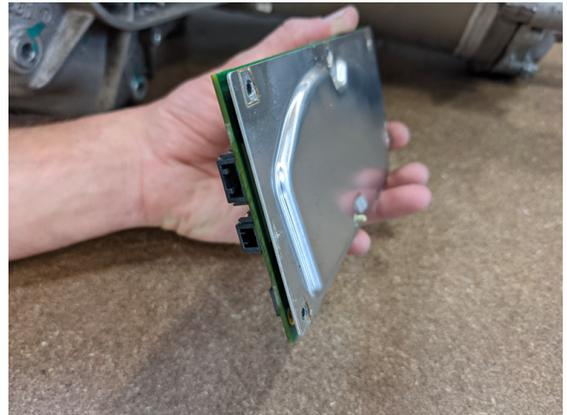
Remove the remaining screw, remove the Tesla board, put the AEM Control Board in place, and secure with the one hold down screw. Line up the other Control Board mounting holes with the EMI shield and then lightly snug up the screw. This will allow adjustment of the Control Board and shield while remounting.
