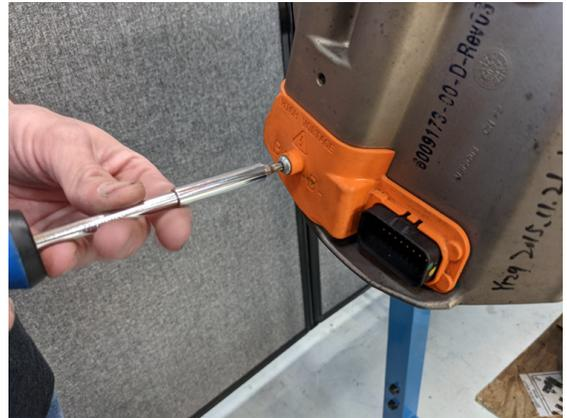
Behind the cover are two rubber o-rings that seal passageways. Carefully pry the cover away to disengage the o-rings and then fully remove cover.
