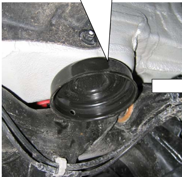
Oberer Original Federteller entfernen. Remove the standard supporting bearing
