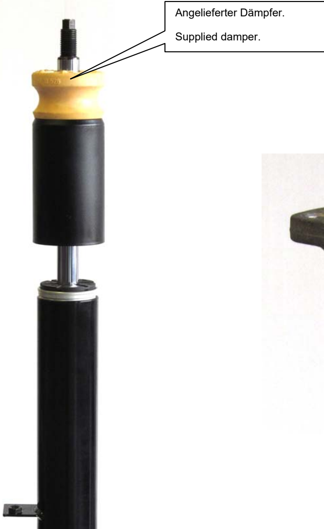
Oberer Original Federteller entfernen. Remove the standard supporting bearing
