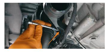
**6.** From the top side of the engine bay, remove the air intake from the vehicle to get better access to the stock hot side pipe.
