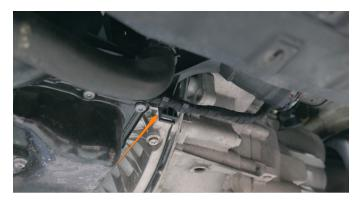
**4.** Using panel clip pliers or a flathead screwdriver, remove the tree clip holding the hose to the stock hot side pipe.
