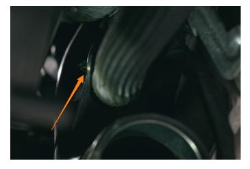
**5.** Using a T30 Torx bit, unbolt the bolt securing the stock hot side pipe to the engine. This is a captive bolt and will remain attached to the pipe.
