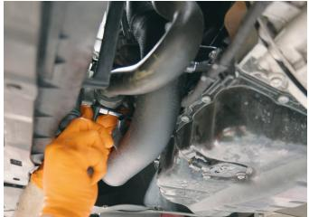
**11.** Unplug the connector from the MAP sensor on the stock cold side pipe by pulling out the lock and depressing the clip on the connector.
