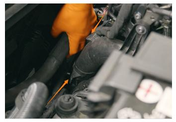
8. Using a T30 Torx bit, unbolt the bolt securing the stock hot side pipe to the bracket on the upper part of the engine. This is a captive bolt and will remain attached to the pipe.
