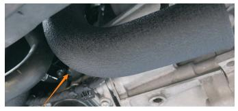
**23.** Using the supplied tree clip zip tie, secure the wiring harness to the cold side pipe. The tree clip can be inserted into the hole on the cold side pipe bracket.
