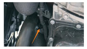
24. Using an 8mm socket or flathead screwdriver, secure the end of the coupler labeled "intercooler in" to the inlet of the intercooler and the end labeled "hot side pipe" to the pipe with two (2) of the supplied 52-76mm worm gear clamps.
