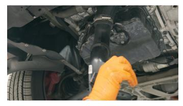
16. Transfer the grommets and captive bolts from the stock pipes to the Mishimoto pipes by pulling the bolt assembly out of the grommet and then removing the grommet from the brackets on the pipes. Next, insert the grommet from the back side of each of the Mishimoto brackets and insert the bolt assembly into the grommet from the front side.
