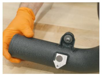
17. Using a T25 Torx bit, remove the bolt securing the MAP sensor to the stock cold side pipe. Then remove the MAP sensor from the pipe and install it into the sensor port on the Mishimoto cold side pipe. Secure the MAP sensor to the Mishimoto pipe using the supplied M6 button head bolt. Tighten with a 3mm Allen key.
