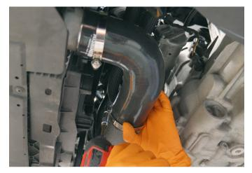
**25.** Install the turbocharger coupler to the turbo outlet and the Mishimoto hot side pipe. Secure the end of the coupler to the turbocharger using the supplied 33-57mm worm gear clamp and secure the other end of the coupler to the hot side pipe using the remaining supplied 52-76mm worm gear clamp. Tighten the clamps using an 8mm socket or flathead screwdriver. (Image on next page)
