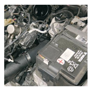
**26.** Using a 10mm socket and the supplied M6 hex head bolt, attached the supplied bracket to the Mishimoto hot side pipe. Then using a T30 Torx bit, secure the bracket to the engine with the one (1) captive bolt that was transferred to the Mishimoto bracket.
