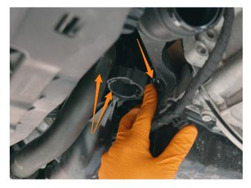
**13.** Using a T30 Torx bit, unbolt the other bolt securing the stock cold side pipe to the engine. This bolt is located behind the MAP sensor. This is a captive bolt and will remain attached to the pipe.
