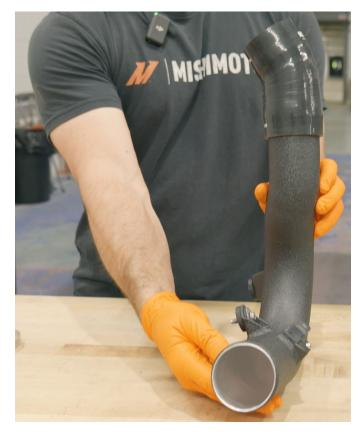
**19.** Install the Mishimoto cold side pipe onto the vehicle up from the bottom of the engine bay positioning the coupler onto the throttle body. Then, using an 8mm socket or flathead screwdriver, secure the coupler to the throttle body by tightening the clamp that was left loose in the previous step.
