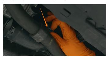
12. Remove the hose from the plastic clip on the stock cold side pipe. Then, using a T30 Torx bit, unbolt the bolt securing the stock cold side pipe to the engine. This is a captive bolt and will remain attached to the pipe.
