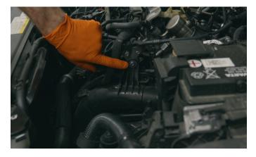
**9.** Using a 7mm socket or flathead screwdriver, loosen the stock hose clamps securing the coupler between the turbocharger and the stock hot side pipe and remove the coupler from the vehicle.
