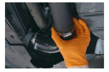
22. Install the Mishimoto hot side pipe onto the vehicle up from the bottom of the engine bay. Then, using a T30 Torx bit, tighten the one (1) captive bolt that was transferred to the Mishimoto hot side pipe to secure it to the engine.
