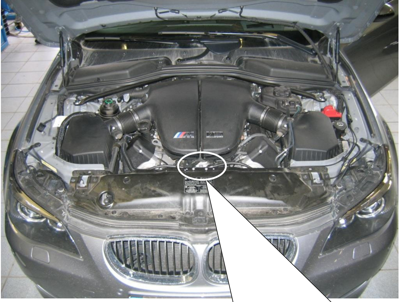
Montageort VA Elektronik Satz / Assembly area front axle electronic kit
