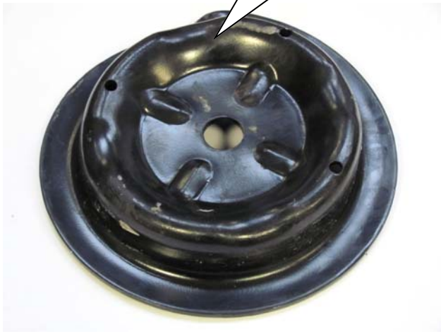
Stahlfederteller Steel spring perch.
