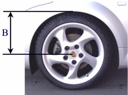
Measurement B Wheel hub center wheel arch
