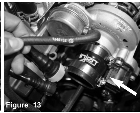
Figure 13 Install the 2" hose to the turbo with clamps provided.
