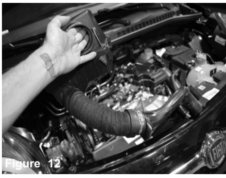
Figure 12 Now lift up and remove the whole intake assembly out of vehicle.
