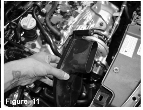
Figure 8 A) Pull back the tube from turbo. B) Disconnect the vacuum line from the fitting on intake tube.
