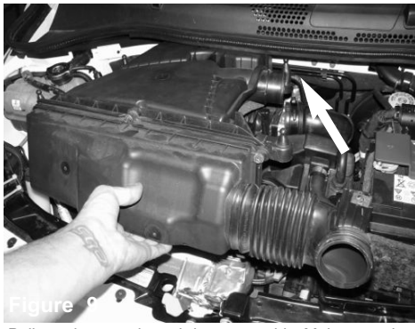
With 8mm socket or nut driver, loosen the bolt holding in the 90 degree plastic snorkel.
