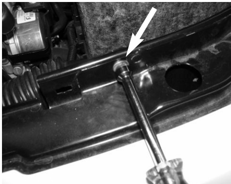
With 8mm socket or nut driver, loosen the bolt holding in the 90 degree plastic snorkel.
