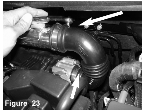
Figure 20 Now secure the 15.9mm hose to the fitting on the intake tube.
