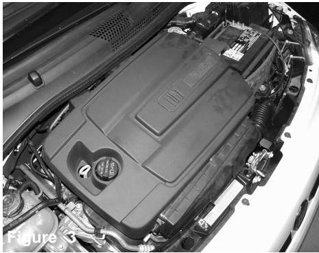
Figure 4 Lift up the engine cover, and remove.
