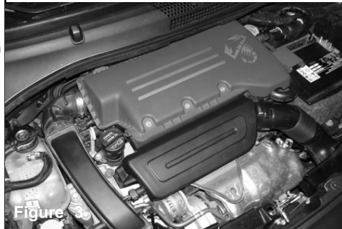
Figure 3 Stock air box assembly shown in this picture. Disconnect battery before the install.
