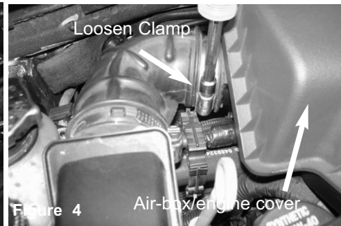
Figure 4 Loosen the clamp on the upper part of the air-box/engine cover using 8mm nut driver.
