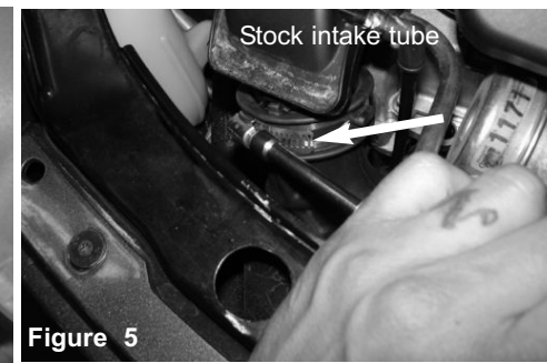
Figure 5 Loosen the clamp on the turbo side of the stock intake tube.
