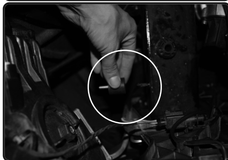
9. Now install the provided M6 vibramount to the threaded stud on vehicle frame. Secure and tighten.
