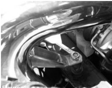
Figure 25 Tighten the nut using 10mm wrench.
