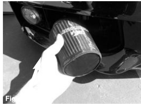
Figure 22 Install the intake tube into vehicle.
