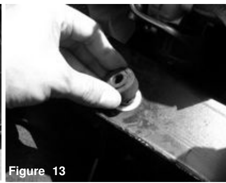
Figure 14 Install the M6 stand off stud to the grommet and push down.
