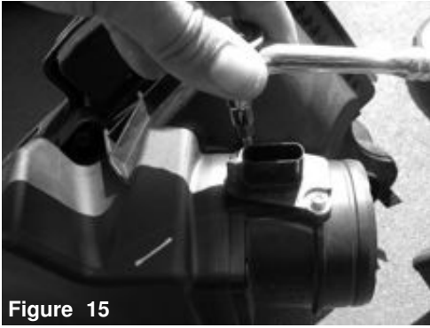
Figure 16 Carefully remove the MAF sensor.
