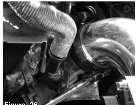
Figure 26 Tighten the remaining clamp using 8mm nut driver.
