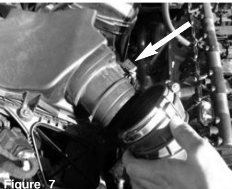
Figure 7 Pull back the factory intake tube.
