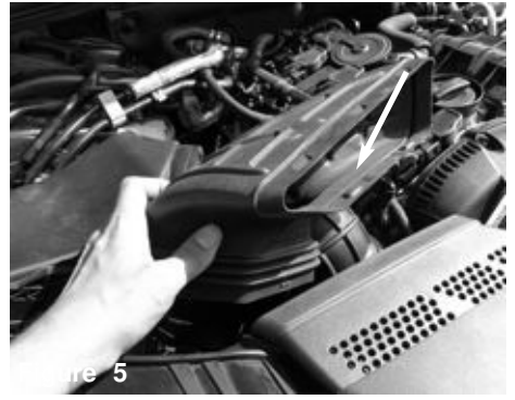
Figure 4 Disconnect MAF sensor harness and set aside.
