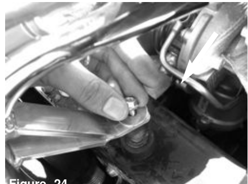
Figure 24 Secure the bracket using provided M6 washer and nut.
