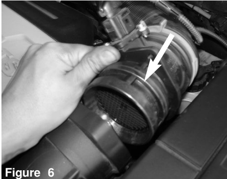
Figure 6 Pull back the MAF sensor and set back.
