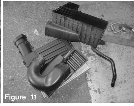
Figure 11 Complete OEM air box removed.
