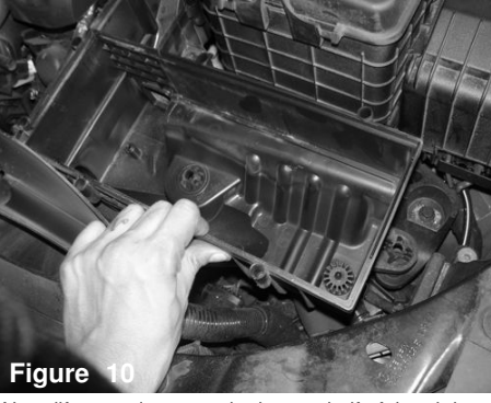
Figure 10 Now, lift up and remove the bottom half of the air box.
