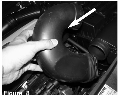
Figure 8 With pliers, carefully pinch clamp and pull intake tube away from air box.
