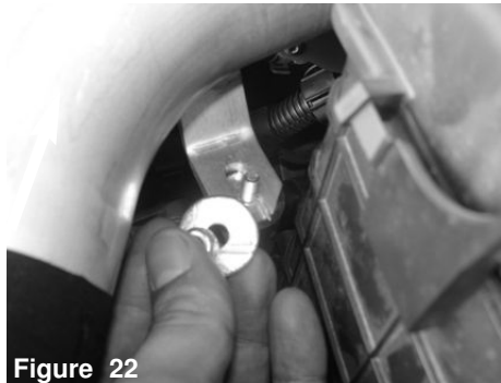
Figure 22 Secure the bracket on intake tube using provided M6 washer and nut.
