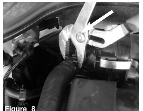
Figure 8 With pliers, carefully pinch clamp and pull intake tube away from air box.
