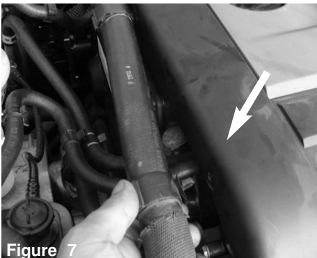
Figure 7 Pull back the diverter tube from air box/engine cover.
