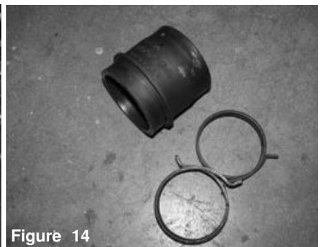
Figure 14 Remove complete stock turbo coupler and clamps shown above.
