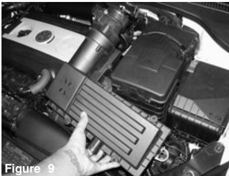
Figure 9 Pull out the complete air box assembly.
