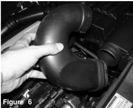
Figure 6 Pull out ram air elbow from air box.
