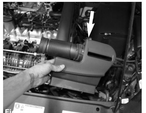
Figure 8 Pull back the ram scoop out of the vehicle.
