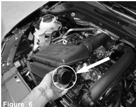
Figure 6 With pliers or channel locks, loosen the clamp on stock ram scoop. Pull back from the ram scoop. Lift up and remove the factory air box.
