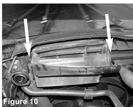
Figure 10 With T25 torx bit loosen the 2 screws holding in the factory ram scoop and remove. Save screws for later install.
