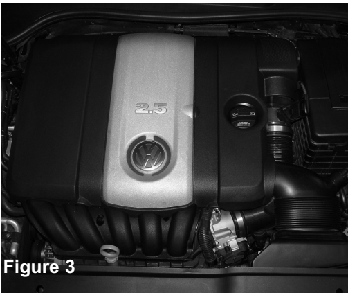
Figure 3 Picture of factory air intake system
