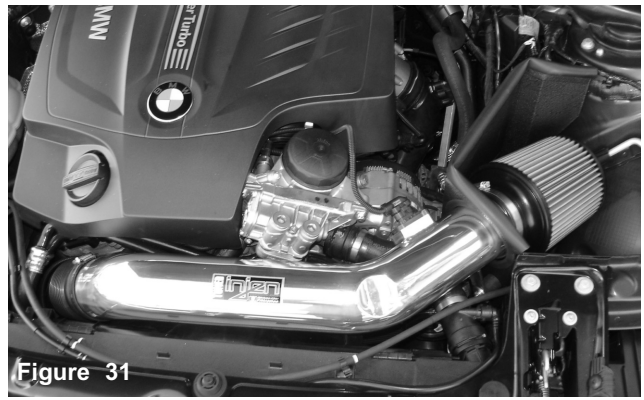
Figure 29 Connect the vacuum line to the fitting on the intake tube. If manual transmission, attach the vinyl cap to the fitting and cap off.
