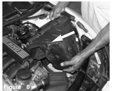
Figure 5 The hose clamp on the air intake duct connected air box cleaner is loosened.
