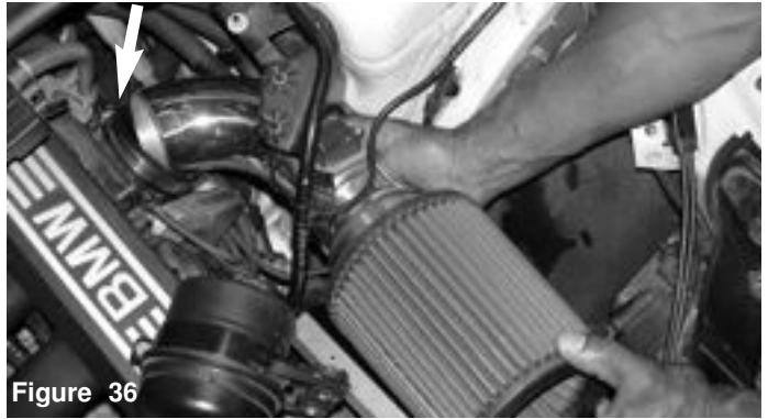
Figure 35 The assembled intake and filter is now lowered into the engine compartment.
