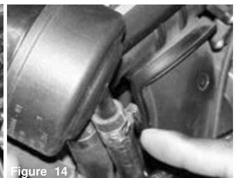
Figure 11 Without disconnecting the two lines, remove the reservoir bottle from the two studs.
