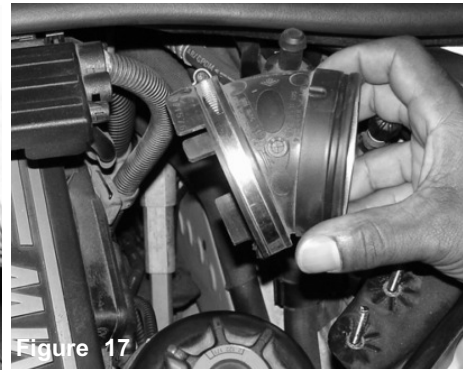
Figure 17 Once you have loosened the clamp, continue to pull the plastic elbow from the throttle body.
