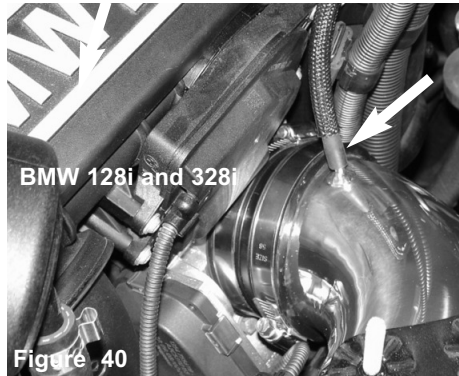
BMW 128i and 328i Figure 39 Installation on the 128i and the 328i: The vacuum hose is pressed over the 5mm intake vacuum port.
