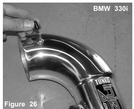
Figure 26 For installation on the 2006 330i, press the supplied 5mm vacuum cap over the 5mm intake port. This intake port is not used on the 330i. Note, there are some 330i that come equipped with the vacuum line.
