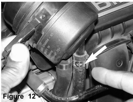
Figure 12 Note: This clamp will not be removed. The clamp will be rotated so that it will not interfere with the air intake.
