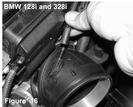
Figure 16 On the 2008-09 128i and 2007-09 328i the vacuum hose is removed prior to loosening the clamp over the throttle body.
