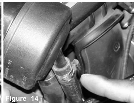
Figure 14 The clamp is now in the correct position, facing to the side. This will prevent any damage to the intake.
