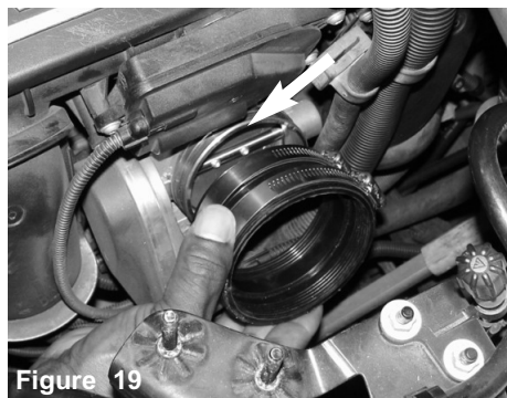
Figure 19 With the power-bands on the step hose, align the step hose over the throttle body.
