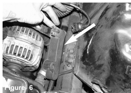
Figure 6 Remove the rubber isolator from the vehicle frame near the alternator
