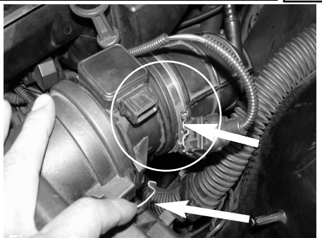
Figure 2 Disconnect MAF sensor harness. Un-clip the air box from the MAF sensor. Pull back MAF sensor from the air box.
