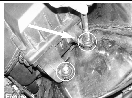
Figure 3 Loosen the 2-10mm bolts holding in the air box.
