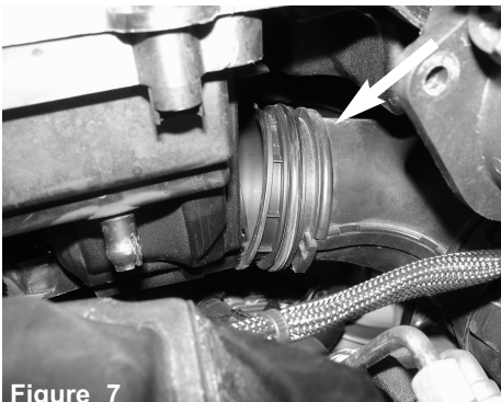
Figure 7 Pull back the snorkel/ram air plastic piece from the bottom half of the airbox.
