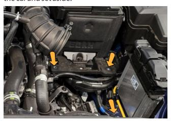
3) Remove the recirc hose ( ) and vacuum hose ( ) from the factory valve:
