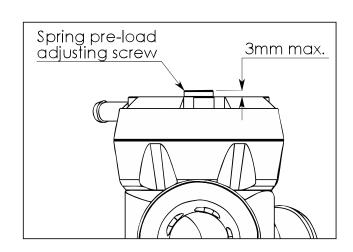
Start by setting the venting bias adjustment to full atmosphere (so you can hear the valve venting during setup), then set the spring pre-load screw level with the top of the valve.
