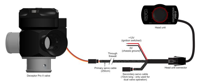
Feed the primary servo cable through the firewall into the engine bay. Ensure that the cable is protected where is passes through the firewall to prevent shorting out.
