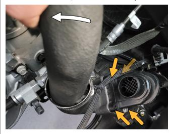
6) Install the GFB valve using the supplied screws and shortened 5mm hex key. It's easiest to start with the screw beneath the electric motor:
