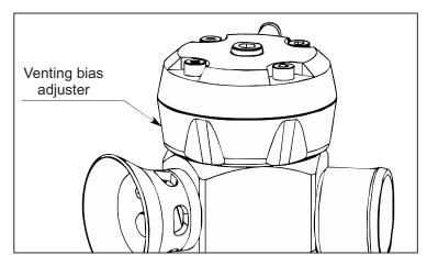
operation (you may still hear the recirc venting if you have an aftermarket intake fitted). You can set the adjustment anywhere in between for a variable venting ratio and to control the sound volume.
