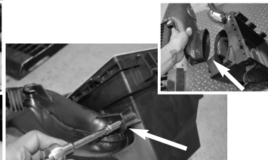
Figure 13 Loosen the screw holding in the factory scoop on the air box. This will be used in the new intake kit.
