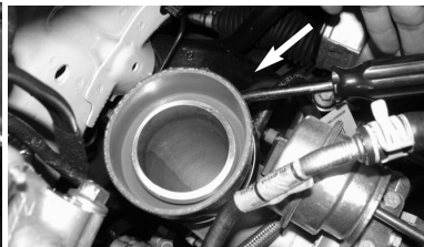
Figure 18 Tighten the clamp on the turbo only. Place clamp on the 3" side in a spot allowing for easy access when you tighten the clamp.
