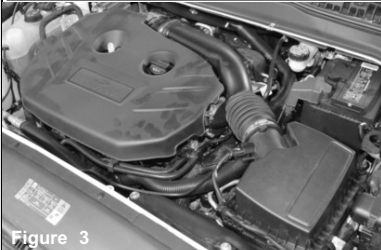
Figure 3 Stock air box assembly shown in this picture. Disconnect battery before the install. Remove the engine cover.
