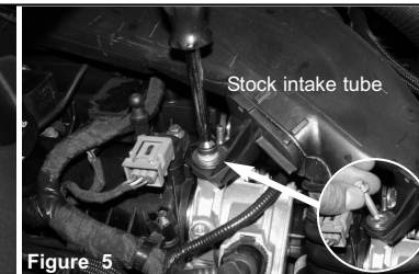
Figure 5 Locate the screw holding in the upper half of the stock intake tube. Loosen using 8mm nut driver or socket. Remove the screw.
