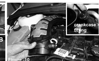
Figure 10 Loosen the clamp on the turbo side, remove the plastic turbo elbow. Disconnect the crankcase line.
