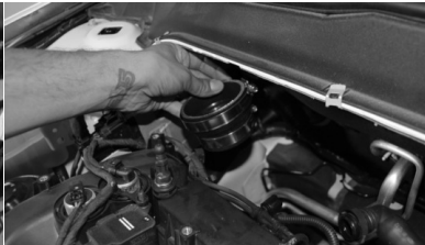
Figure 17 Install the step hose to the turbo with clamps provided.
