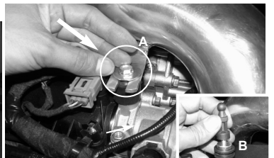
Figure 20 A) Install the primary intake tube and secure to the turbo and bracket to the vibramount. Secure using provided m6 nut and fender washer. B) Re-install the fitting from step 9, this will allow for the engine cover install.
