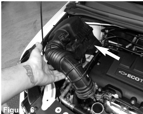
Figure 6 Pull out the air box from the side of the vehicle. lift up and pull the intake assembly out of the vehicle.
