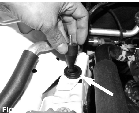
Figure 7 With oil or lubricant, place some on the factory grommet located where the factory air box mounted too. Now install the M6 stand off stud.
