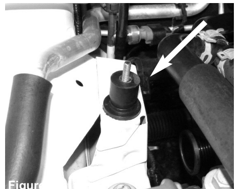
Figure 8 Secure the stand off stud so it seats tightly.
