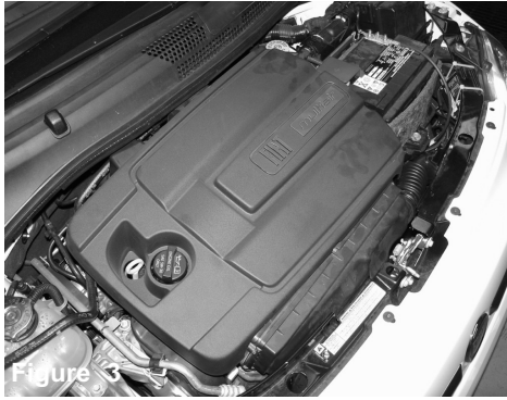
Figure 4 Lift up the engine cover, and remove.
