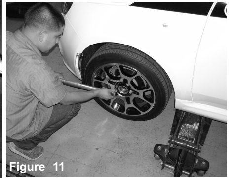
Figure 11 Carefully jack the front driver side of vehicle, and loosen the bolts on the front wheel and remove. This will allow for easier installation. Note: Make sure the vehicle is secure!
