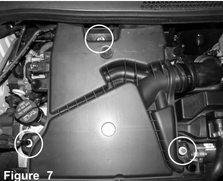
Figure 7 Loosen the 3 bolts holding in the air box using 8mm socket or nut driver.
