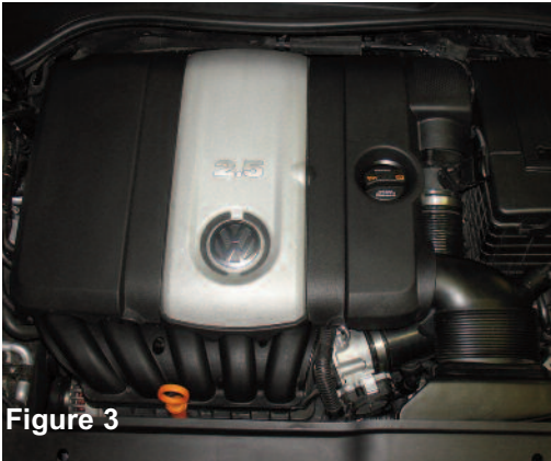
Figure 3 Picture of factory air intake system
