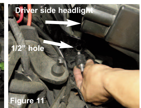
Figure 11 Place the M8 vibramount into the 1/2" hole located on the frame under the driver side headlight. Use the headlight in the photo for reference. Use a 3/8" washer and M8 nut to secure the vibramount to the chassis
