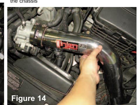
Figure 14 Drop the intake tube into the engine bay and put the filter end of the pipe into the bumper cavity under the driverside headlight. Position the other end into the 3.0" coupler on the throttle body
