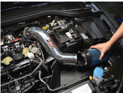
23. Install the air filter to the intake tube and secure using the provided clamp.
