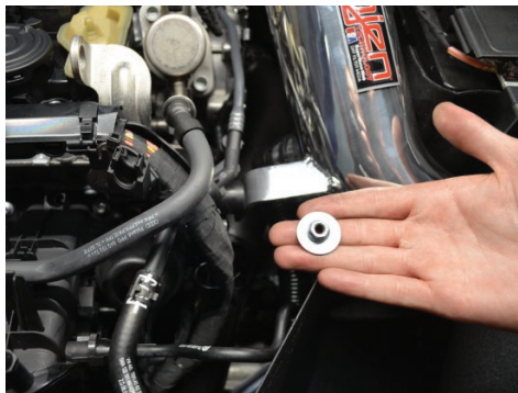
21. Bolt down the intake tube using the provided M6 nuts and washers.
