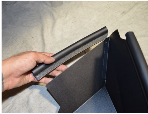
14. Install the 9.5" bulb trim onto the front edge of the heat shield. Trim the bulb trim if necessary.
