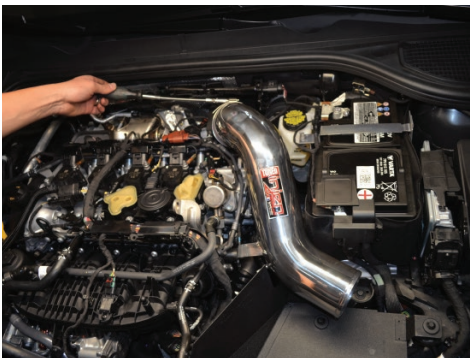
20. Install the intake tube and line up the bracket to the M6 Vibra mount.
