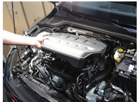
9. Remove the engine cover from the engine bay.
