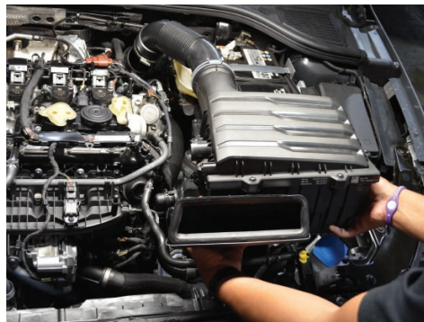
8. Remove the intake assembly from the engine bay. Note: Grommets are attached to the air box, apply lubricant if necessary.
