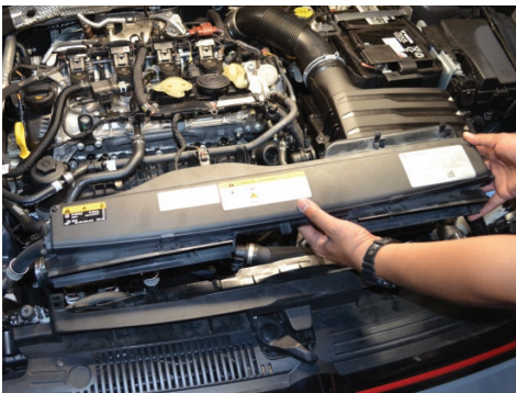
7. Remove the front scoop from the engine bay.
