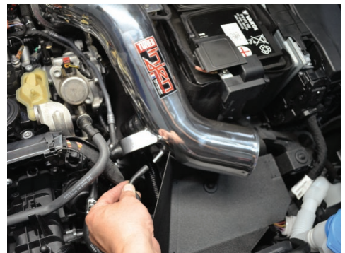
22. Connect the vacuum line to the intake tube.
