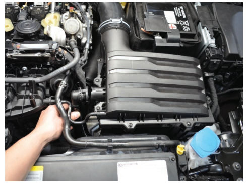
3. Squeeze the retaining tabs on the secondary air injection tube and pull away from the air box.
