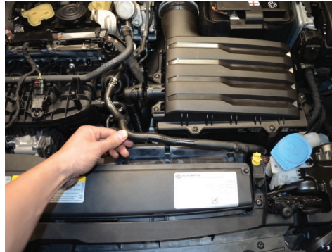
5. Detach the coolant line from the front scoop.
