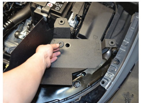
12. Install the three grommets to the bracket holding the stock charge pipe.
