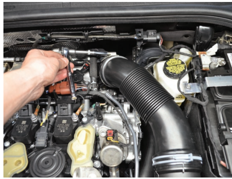
2. Loosen the clamp holding the stock intake tube to the turbo inlet.
