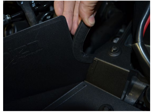
15. Install the 5" bulb trim onto the side edge of the heatshield. Trim the bulb trim if necessary.
