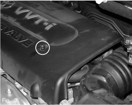
Fig. 3 Remove the engine cover that is secured by two 6mm acorn nuts.
