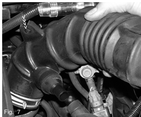
Fig. 7 Unclip the vacuum hose from the small rubber jaw like holder used to secure the entire vacuum hose in place.
