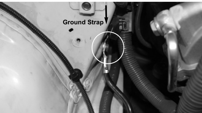
Now move to new location behind the strut tower. Locate the threaded insert and secure and tighten the ground wire.
