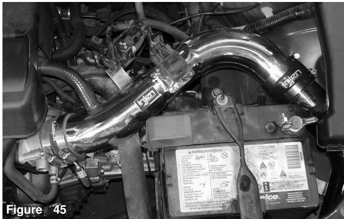
Figure 45 align the entire intake for best possible fit. Once you have established the best fit, free from any moving parts, continue to tighten all nuts, bolts and clamps.
