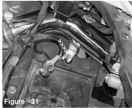
Figure 31 The secondary intake is in the resonator opening while the intake bracket sits flush over the vibra-mount stud.
