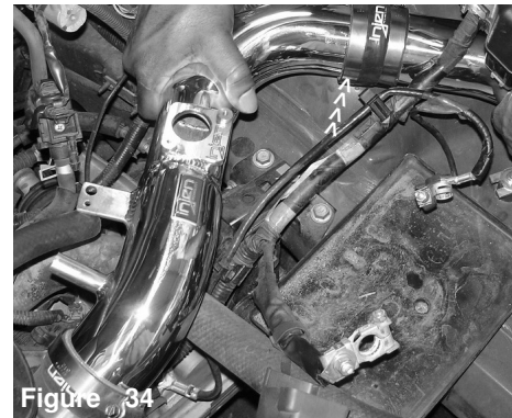
Figure 34 The intake is in the throttle body step hose and the intake is pressed into the secondary intake straight hose.
