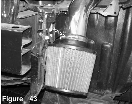
Figure 43 Once the intake end is butted up to the filter stops, continue to tighten the filter clamp.
