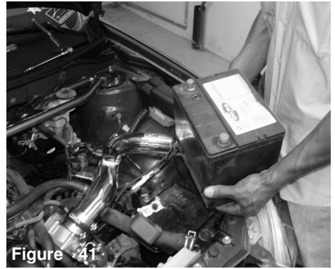
Figure 41 Once you have installed the intake, continue to re-install the battery back to its original location.
