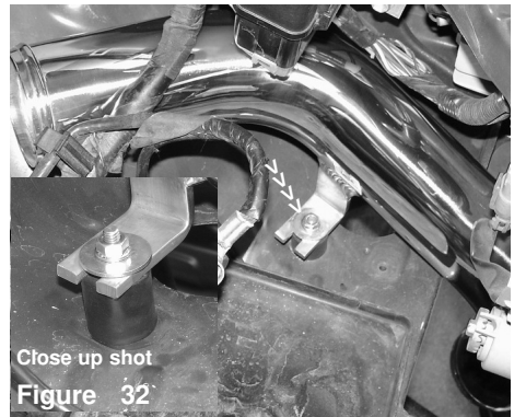
Close up shot Figure 32 The m6 flange nut and fender washer is used to secure the secondary intake.
