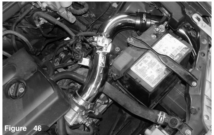
Figure 46 Once the intake has been aligned and proper clearance has been made throughout the length of the intake, start the engine and listen for possible air leaks, rattles or rubbing. If any of the above are heard, go back and re-adjust the intake and check all fittings, clamps and bolts.
