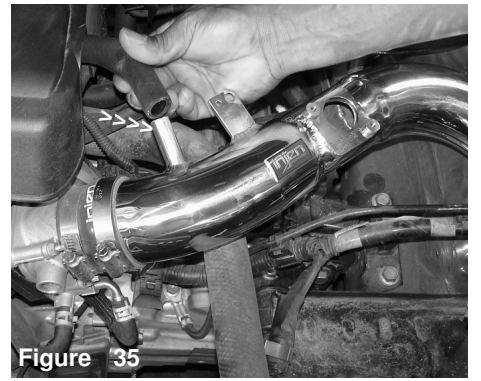
Figure 35 Press the other end of the 17mm heater hose over the intake port as shown above.
