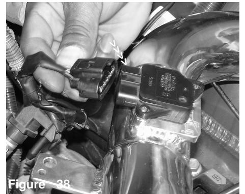
Figure 38 Press the electrical harness clip to the mass air flow sensor until it snaps in place.
