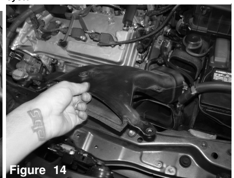
Figure 14 Loosen the 2 bolts holding in the Ram air unit and remove. This will be used again when finished with the install.
