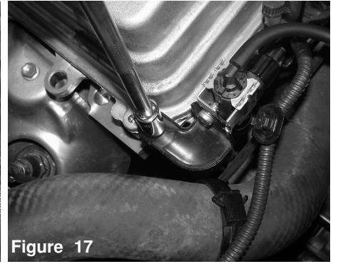
Figure 17 Now secure and tighten using the bolt from step 15. The VAD module is now secured.
