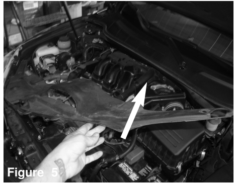
Figure 5 Now remove the front plastic engine cover.
