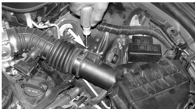
Figure 7 Loosen and remove the two mass air flow sensor bolts.
