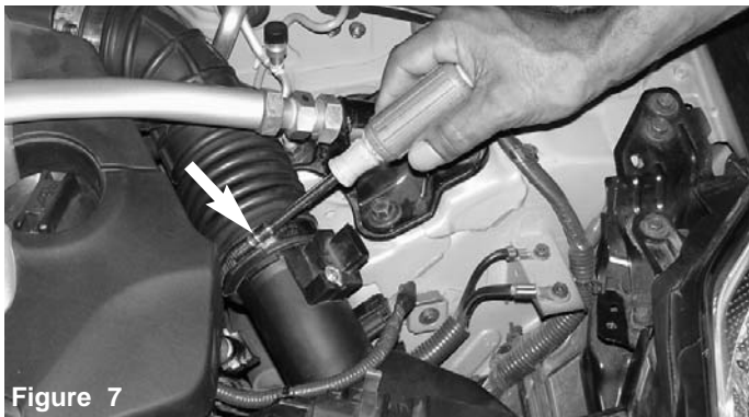
Figure 5 Depress the tab and pull the electrical harness connector from the mass air flow sensor.
