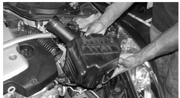
Figure 8 Loosen and remove the two mass air flow sensor bolts.
