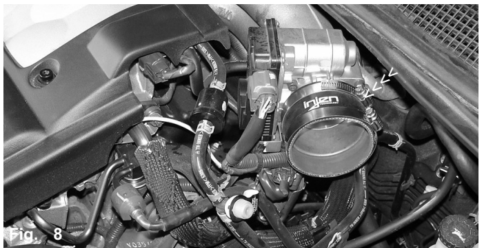
Fig. 8 Press the 3 1/8" straight hose over the throttle body and use two .362 power-bands on the hose. Tighten the band located over the throttle body at this point.
