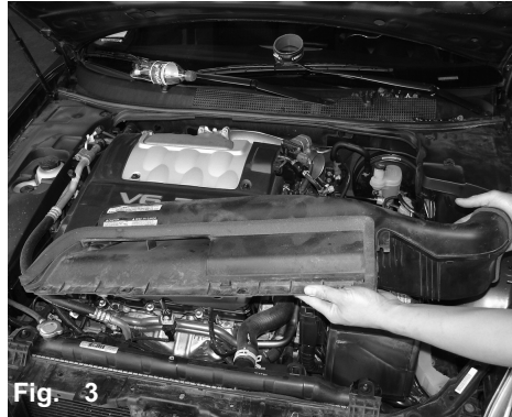
Fig. 3 Remove plastic expanding plugs holding the front air scoop over the radiator. Once all plugs have been removed, continue to remove the air scoop.
