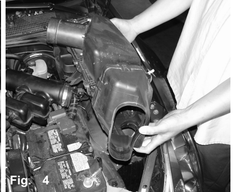
Fig. 4 Loosen clamps and remove bolts from the stock air intake box cleaner in order to remove the entire air cleaning assembly.
