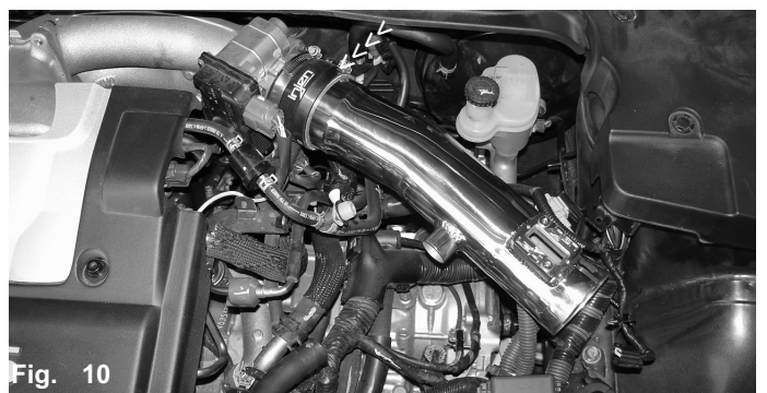
Fig. 10 Insert the top end of the intake into the throttle body hose. Semi-tighten the other power-band just enough to hold the intake in place.
