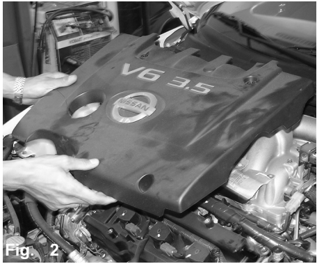
Fig. 2 Remove the four m6 bolts that secure the engine cover over the intake manifold. Once all bolts have been removed, continue to remove the engine cover.
