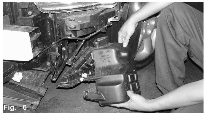
Fig. 6 Once the bumper has been removed continue to disconnect and remove the plastic air intake resonator box.
