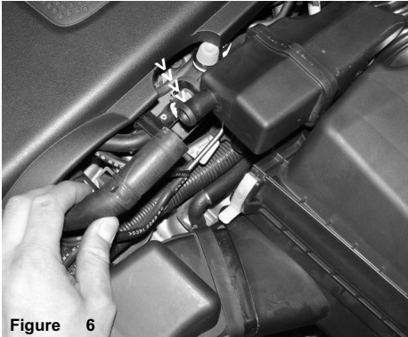
Figure 6 Once the tension clamp is pulled away, continue to pull the hose away from the CCV box.
