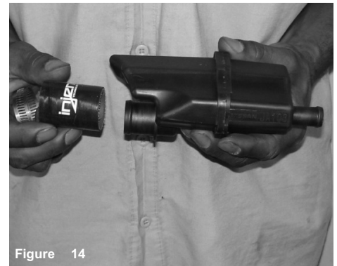
Figure 14 Press the 1/8" straight hose over the CCV box port and use two small clamps.
