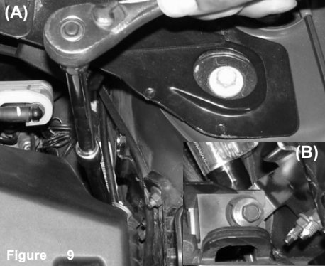
Figure 9 A 10mm socket and ratchet is used to remove an m8 bolt (A). The m8 bolt is located just behind the top air box on the right hand side (B).
