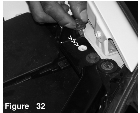
Figure 32 The m8 screw is now removed from the bracket as shown above.
