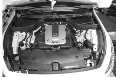
Stock air box assembly shown in this picture. Disconnect battery before the install.
