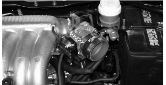
Take the 2 3/4" straight hose and press it over the throttle body, use two clamps and tighten the clamp on the throttle body side.
