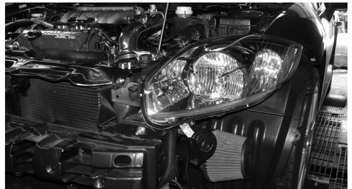
Once the entire cold air intake has been installed, adjust for best possible fit. Once the intake has been cleared from rubbing and rattling continue to tighten all nuts, bolts and clamps. Periodically, check for rubbing, leaks or rattling along the length of the intake in order to avoid damage to the intake.
