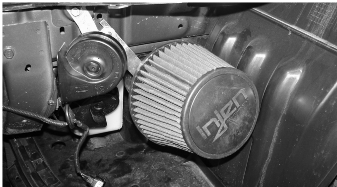
Press the Injen filter over the end of the coupler placed on the silicone intake. Once the filter has been fully pressed into the coupler continue to tighten the filter neck clamp.
