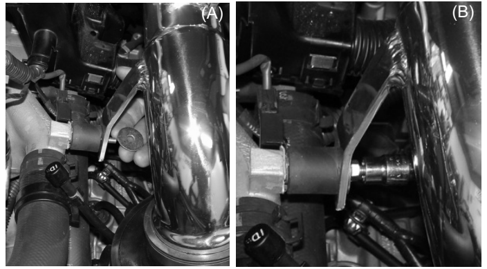
Take the fender washer and place it over the vibra-mount stud (A). Now screw the m6 flange nut on the vibra-mount stud to secure the entire intake (B).
