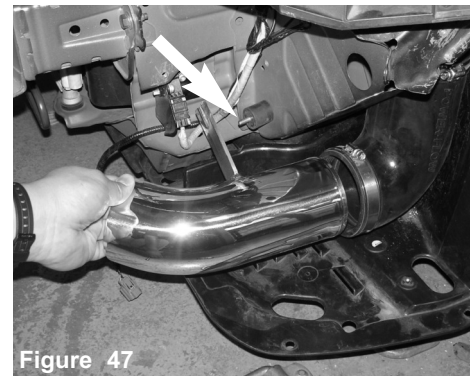
Figure 47 Align the secondary intake to the 90 degree hose, insert the secondary intake into the 90 degree hose. Also make sure the bracket lines up with the vibra mount
