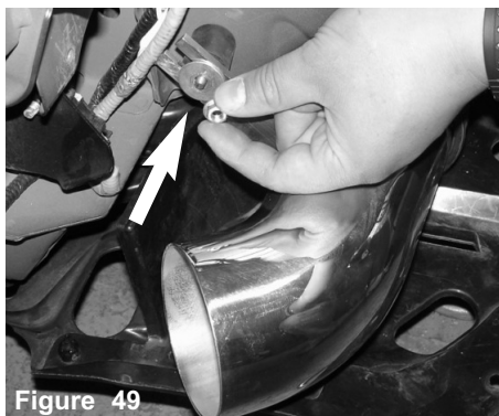
Figure 49 Use the last M6 nut and fender washer to secure the bracket to the vibra mount.
