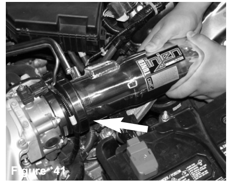
Figure 41 Press the tube with the air mass sensor side into the 2 7/8" X 3 1/4" step hose.
