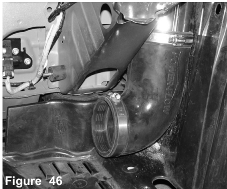
Figure 46 The 90 degree 3 1/2" hose is shown attached to the end of the primary intake.
