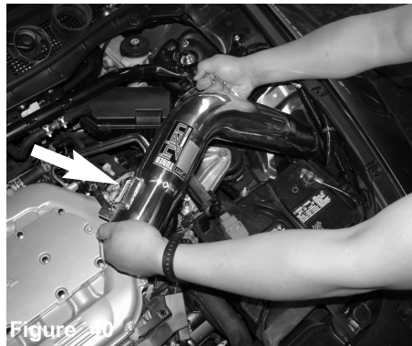
Figure 40 Place the primary tube (longer tube) into the wheel well opening. Make sure the air mass sensor adapter side is on the top side.
