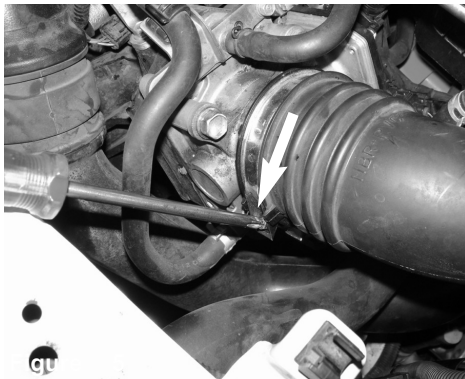
Loosen the clamp on the throttle body using phillips screwdriver.
