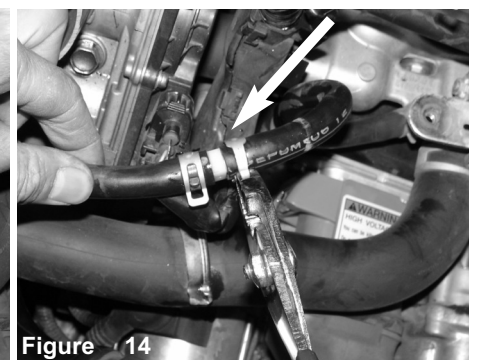
Figure 10 With pliers, pull back the throttle coolant line away from the metal fitting. Pull back line from engine side also.
