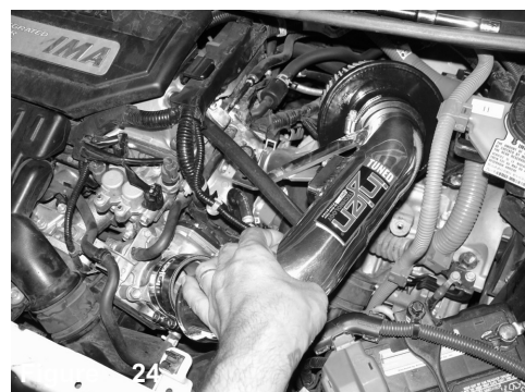
Figure 21 Install the MAF sensor into the new injen intake tube,
