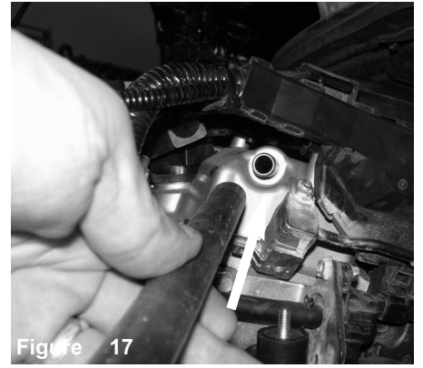
Figure 17 Attach the provided 10mm hose to the engine crank case fitting.
