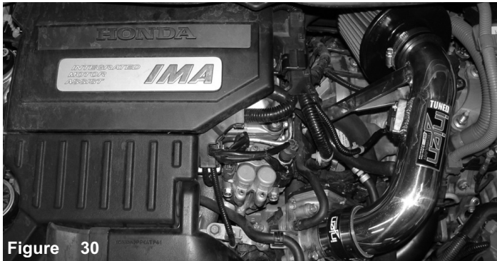
Figure 30 Align the entire intake for the best possible fit. Once you have rechecked and cleared the intake from all moving parts, continue to tighten all nuts, bolts and clamps.
