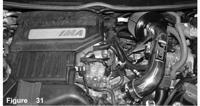
Figure 31 Your intake system install is now complete. Thank you for choosing Injen Technology.
