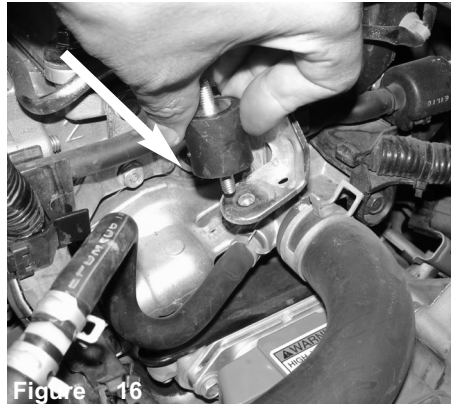
Figure 16 Install the provided M6 vibra mount to the factory mounting point where air box mounted to closes to engine.
