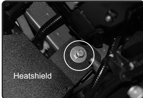
10. Secure the heatshield tab using provided M6 screw and washer.
