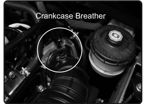
3. With pliers, remove the hard crankcase line out of the intake tube.
