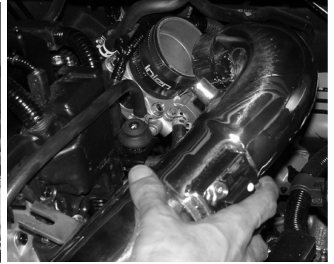
Gently, insert the top end of the intake into the 2 1/2" straight hose located on the throttle body.
