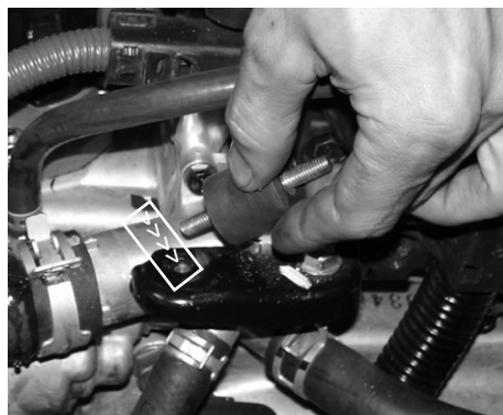
Take the vibra-mount and line it up to the air box brace mounted on the upper coolant outlet housing.
