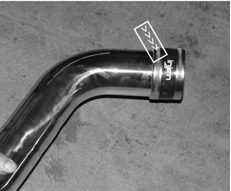
Take the remaining three inch straight hose and press it over the secondary intake. Use two clamps and tighten the clamp located on the intake side.
