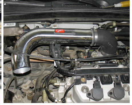
The primary intake is now installed and in place.
