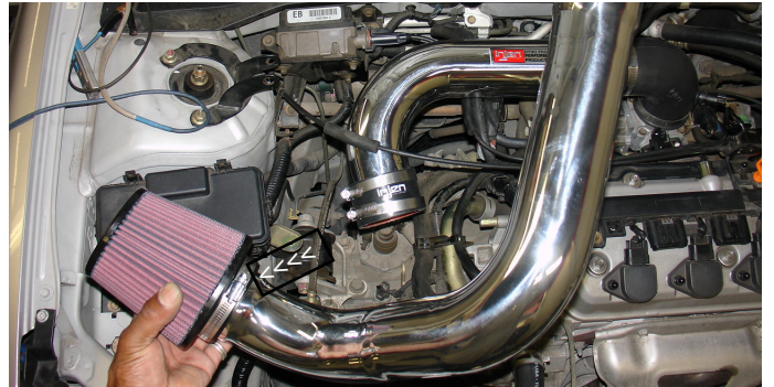
Press the Injen filter over the end of the secondary intake as shown above. Be sure to tighten the clamp on the filter neck.
