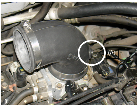
Place the one clamp on each end of the 90 degree elbow. Place the 90 degree elbow over the throttle body then semi-tighten the clamp on the throttle body. Press the grommet into the 3/4" hole in the elbow then press the grommet into the hole (A).
