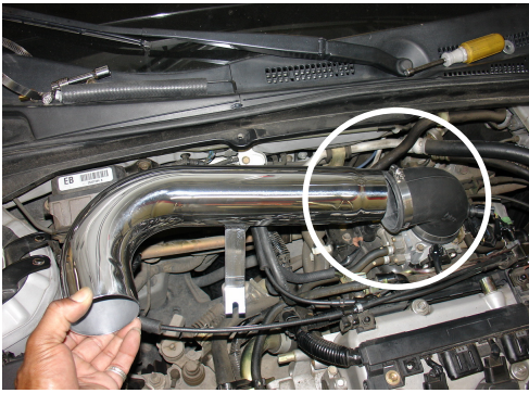
Take the primary intake and press the straight end into the 90 degree elbow as shown in this picture.
